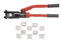
This hydraulic crimper is sturdy and easy to operate, with a strong maximum working pressure of up to 14 tones. It has a Crimping range of 16-300 sq mm and includes 11 crimping dies. With a stroke of up to 22 mm and hexagon type crimping, this handy tool comes complete with a convenient carry case for easy storage and portability.
