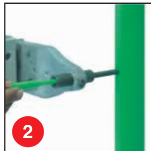
Simultaneously heat the hole section in the pipe line and repair bar using repair section die and welding device for about 5 to 7 seconds depending upon the pipe thickness.
