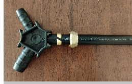
Step 3: Round & Chamfer the pipe (3-5 rotations).
