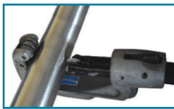
Step 1: Cutting the Tubes
