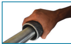
Step 3: Chamfering the Tubes
