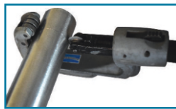
Step 2: Grooving the Tubes
