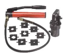
This is a remote control style hydraulic crimping tool. It is intended to crimp AI and Cu connectors from 50-400 sq.mm on cables, can be widely used in electric transmission and distribution work. External hydraulic pump is required to work with the tool. Pump can provide pressurized oil to the tool, operator can install proper dies according to the application, easy, fast and precise crimping can be assured.
