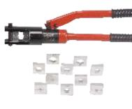
This hydraulic crimper is sturdy and easy to operate, with a strong maximum working pressure of up to 12 tones. It has a Crimping range of 10-120 sq mm and includes 08 crimping dies. With a stroke of up to 14 mm and hexagon type crimping, this handy tool comes complete with a convenient carry case for easy storage and portability.
