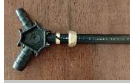
Step 3: Round & Chamfer the pipe (3-5 rotations).
