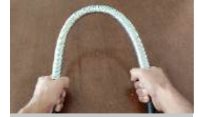
Pipe Bending: Bend pipe using Internal / External bending springs.
